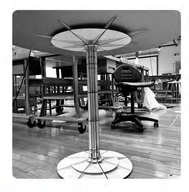
Individual pieces were lazer-cut with plywood and spray painted and assembled by hand
